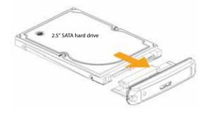
4 Gently slide the drive tray, with drive attached, into the enclosure.
